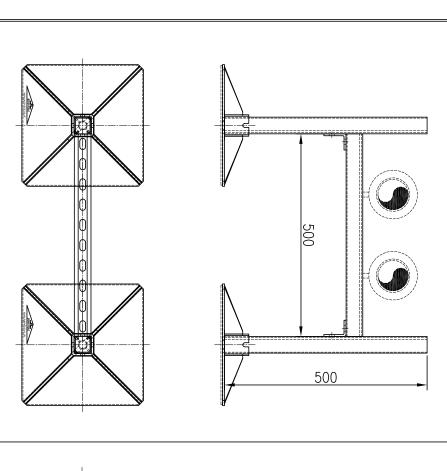
FIRST ANGLE PROJECTION - DO NOT SCALE - IF IN DOUBT ASK - ALL MEASUREMENTS IN MM - REMOVE ALL SHARP EDGES - TOLERANCES UNLESS STATED LINEAR±0.5 TOL/ ANGULAR±0.5 DEG
